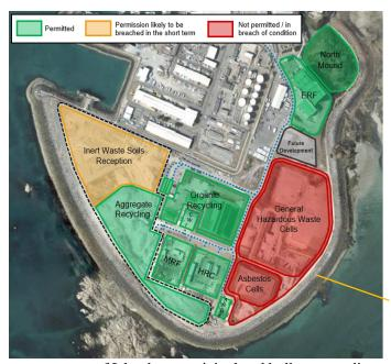
The waste operation at La Collette includes management of municipal and bulky waste through Energy Recycling Facility (ERF), the Clinical Waste Incinerator (CWI). Household Recycling Centre (HRC), Metals Recycling Facility (MRF), organic recycling, aggregate recycling, inert and hazardous waste. waste, including asbestos.
